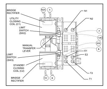
Figure 4. The "W/V-Type" Transfer Mechanism
